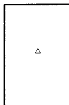
Figure 326. Triangulation Station. The symbol represents a described horizontal control point which is marked on the ground and which was established by triangulation or traverse of third or higher order accuracy.
